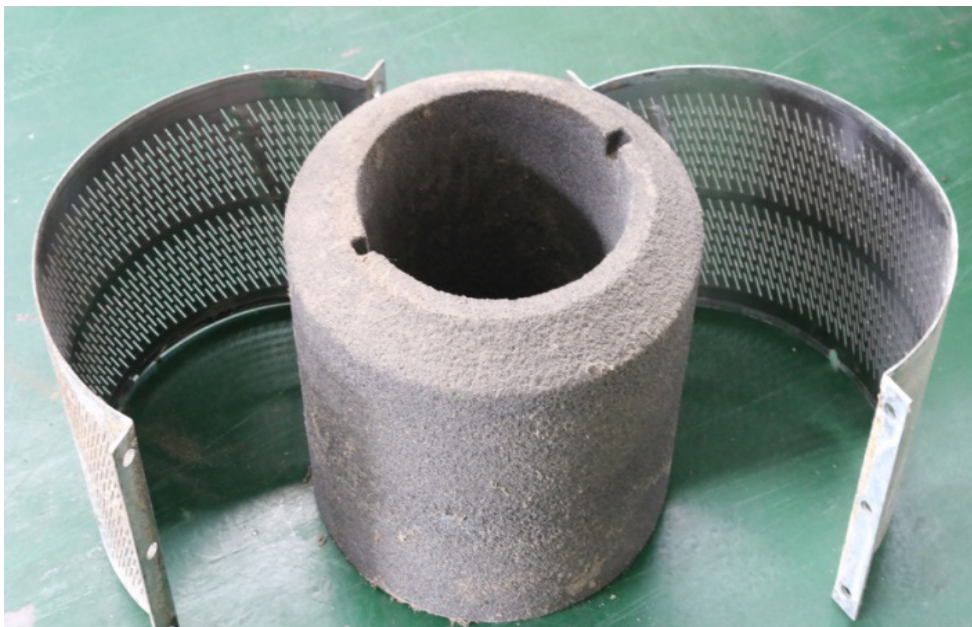
Figure 28. Slotted screen and abrasive stone of a horizontal abrasive whitener
