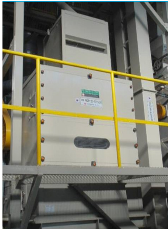
Figure 13. Pre-cleaner with destoner machine
